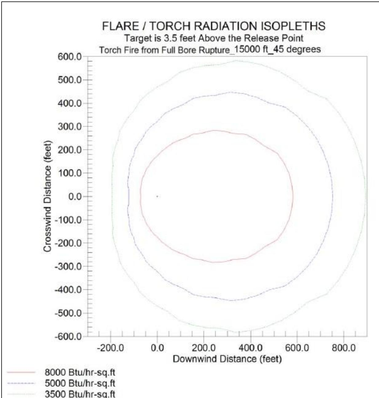
Figure 8-7: Full Diameter Rupture Torch Fire at 45° Release Angle
