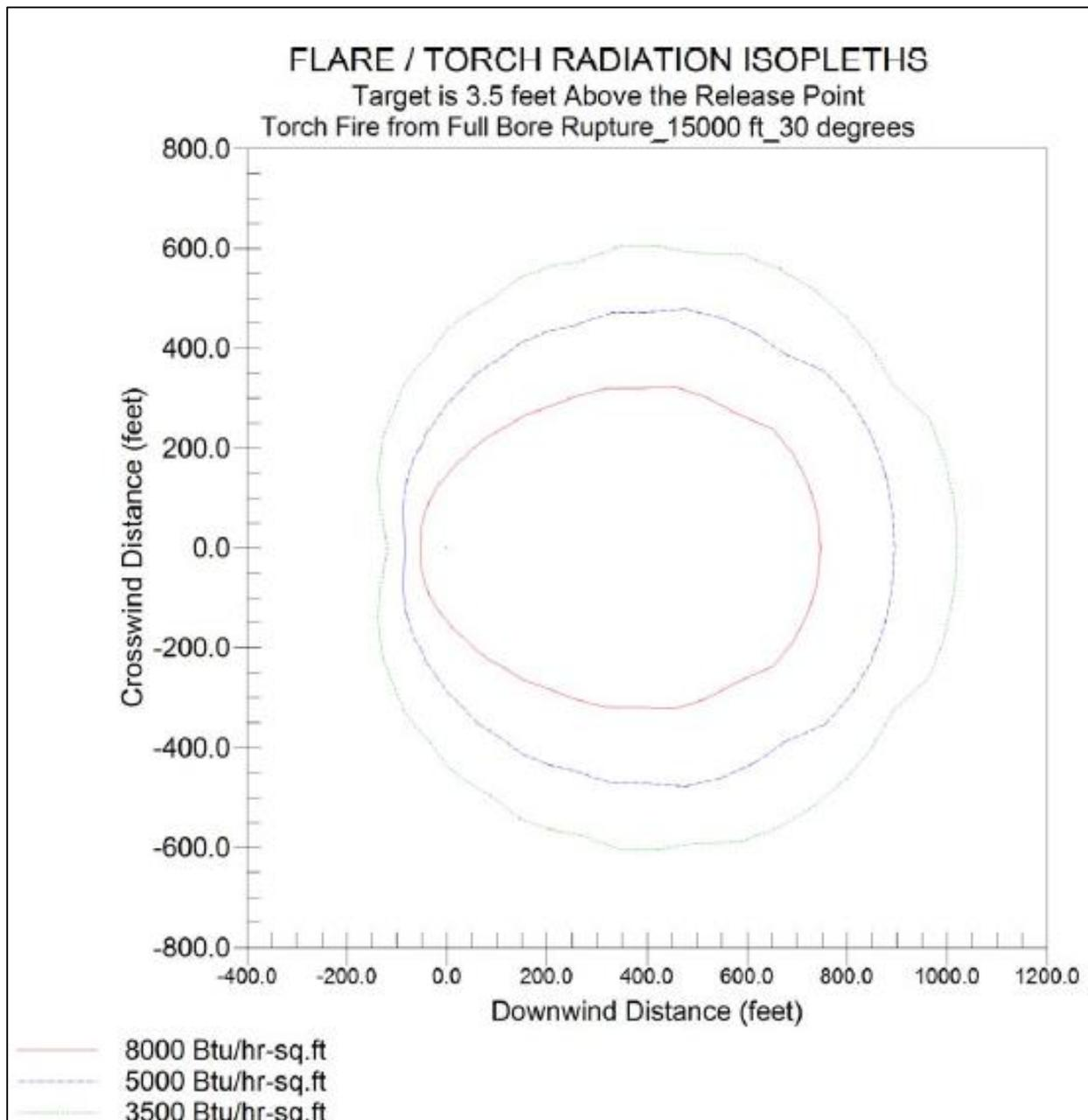
Figure 8-6: Full Diameter Rupture at 30° Release Angle
