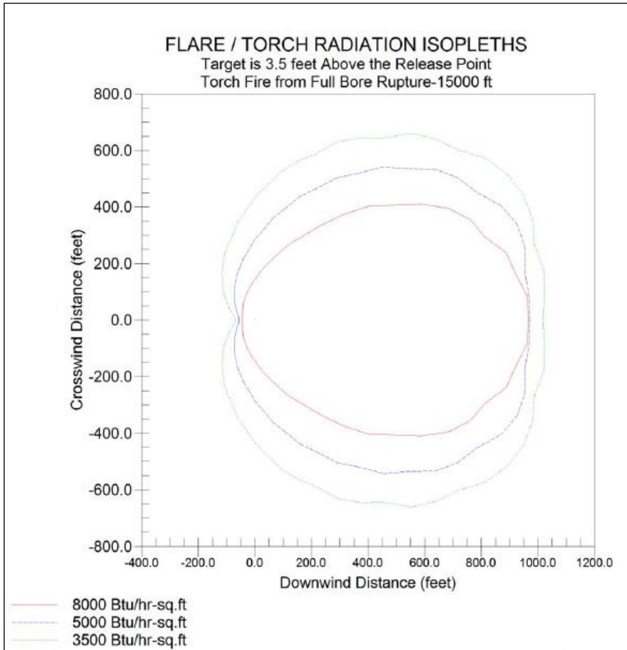
Figure 8-5: Full Diameter Rupture Torch Fire at 0° Release Angle
