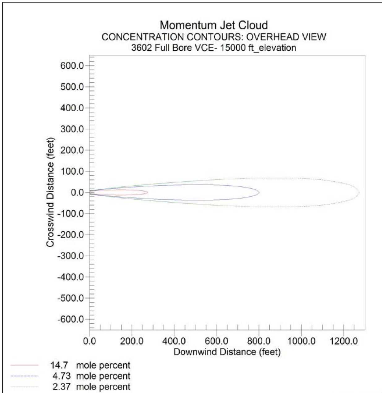
Figure 8-2: Vapor Cloud Dispersion, Full-Diameter Rupture
