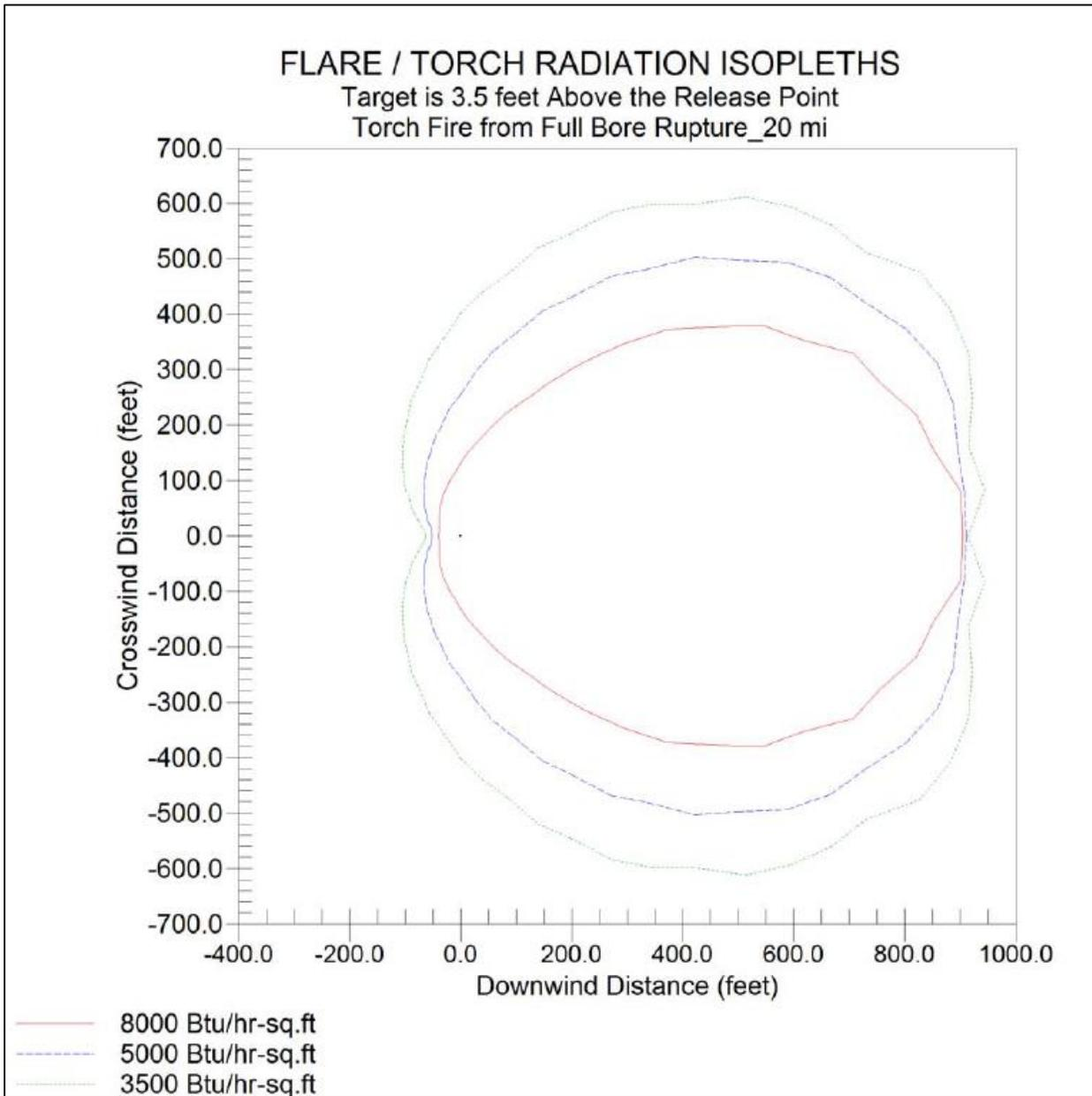
Figure 8-8: Full Diameter Rupture, 20 miles from the Source
