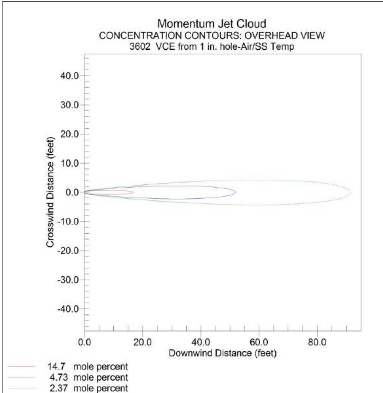
Figure 8-3: Vapor Cloud Dispersion, 1-inch Leak
