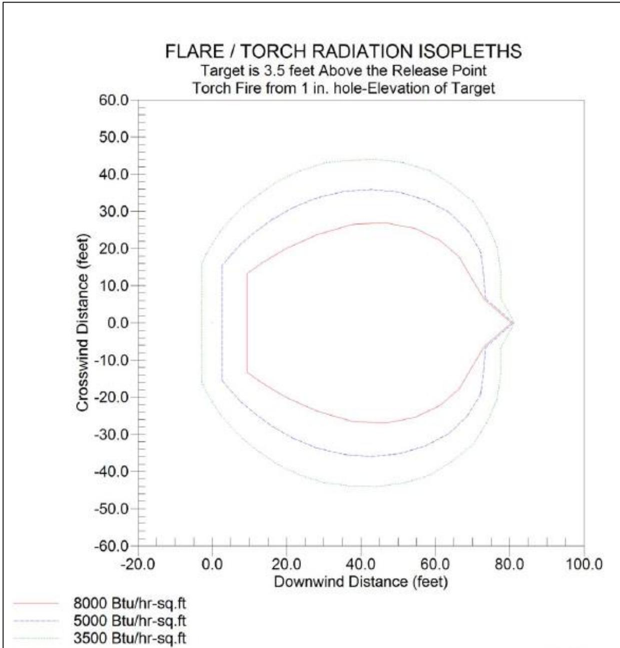
Figure 8-4: 1-inch Leak Torch Fire
